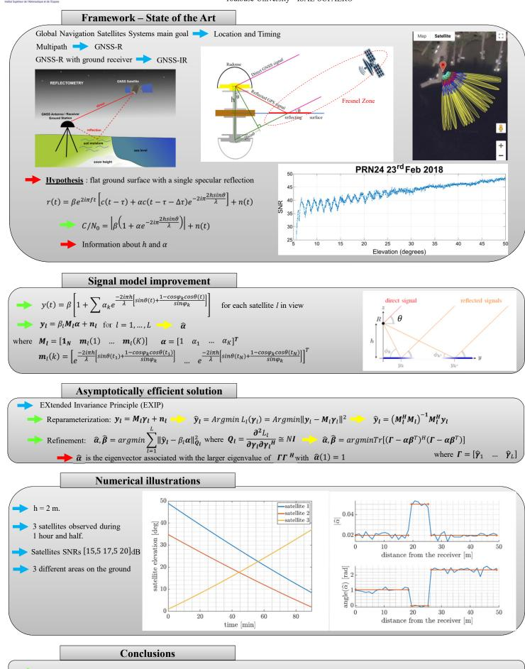
Extended the standard specular GNSS-IR model to provide more precise mapping description.
